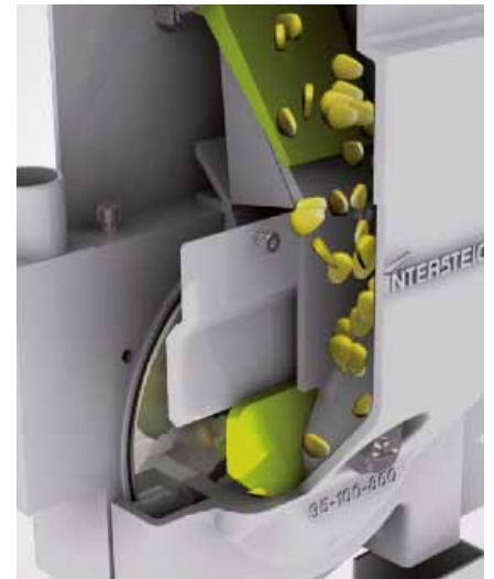
The turning seed chamber in the seed metering unit of the Dynamic Disc
