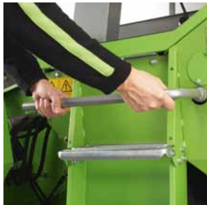
Threshing drum reversing mechanism
