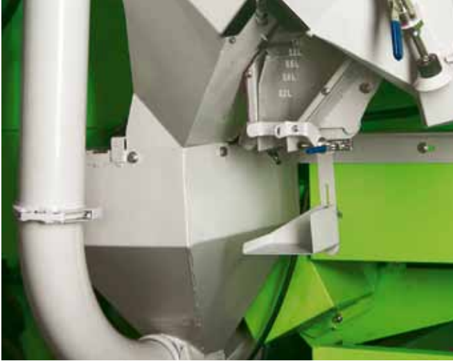
Side mounted sampler (2-man harvesting method)
