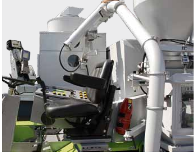
Sampler mounted next to driver's seat (1-man harvesting method)
