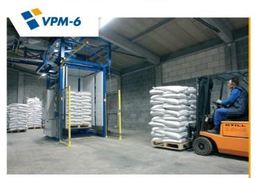
The VPM-6 is a palletizer suitable for packers who require more capacity and set higher standards for the stacking result. The machine is standardly equipped with a three-sided stacking bin enclosing the pallet and ensuring an accurate stack of the product.
